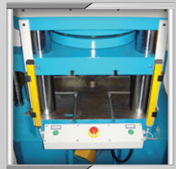
HAND PROTECTION FOR PRESS OPERATION
