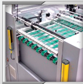
OPERATOR FINGER PROTECTION IN PAPER SORTING MACHINES
