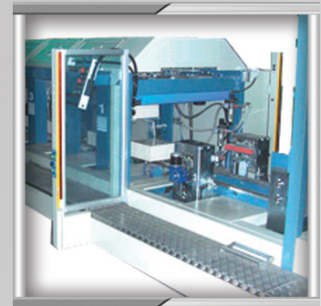
HAND PROTECTION FOR AUTOMATED SORTING MACHINE
