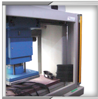
OPERATOR HAND PROTECTION ON PRESS FIXTURE
